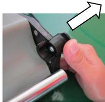
Slide carriage release button to right to release carriage rod
