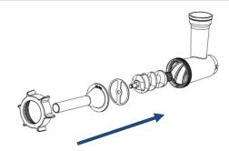
2. Attach the grinder head to the motor housing.
