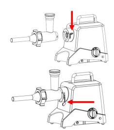
3. Press down the locking handle to make sure that the **grinder head** is locked firmly.
